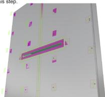
6) Apply joint compound and mesh tape to all seams and the mud-in bead, then let cure
