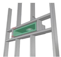
2) Install plenum box per specifications. This example uses straps and spacers to center the plenum box in the frame opening
