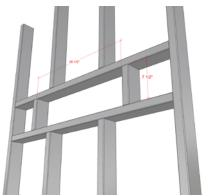
1) Install framing per specifications. This example uses the standard framing specification for a 24" linear diffuser 1 slot x 1", which calls for a 24.5" x 7.5" between framing
