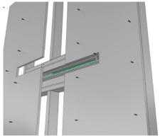
5) Install drywall up to the mud-in bead and secure with screws
