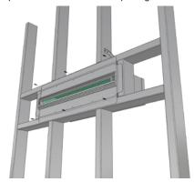
4) Secure diffuser and plenum box to framing. Be sure to connect all ductwork to plenum boxes before moving past this step.
