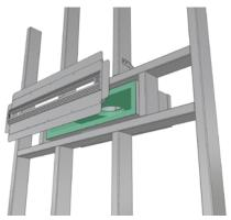
3) Fit diffuser onto plenum box. Sealant or tape may be used in this step to create a tighter seal, if needed.
